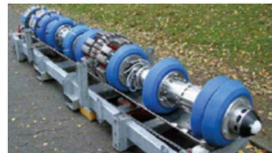
**Developed** an in-house 28-inch inline inspection tool (IPIG) based on **Magnetic Flux Leakage (MFL) technology** for our Pipelines Division.
